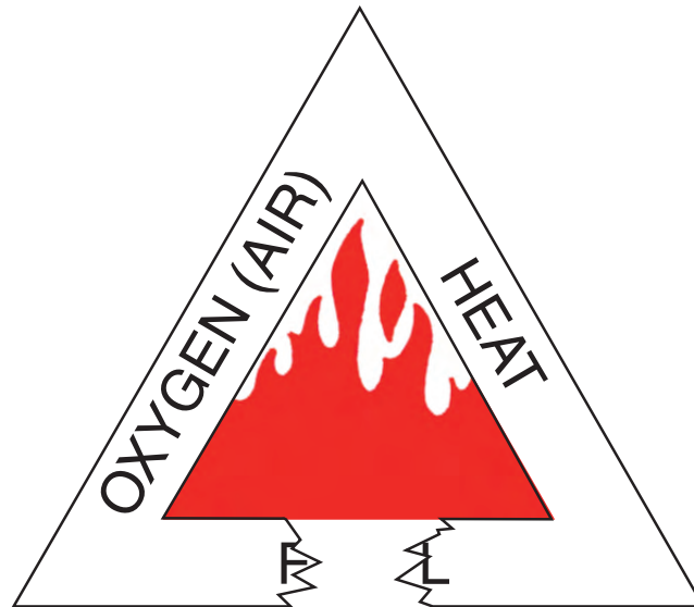
Illustration 2.4 Broken fire triangle (fuel)
