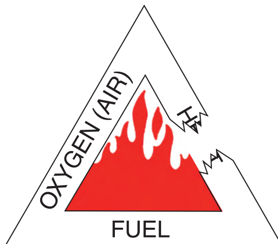
Illustration 2.3 Broken fire triangle (heat)
