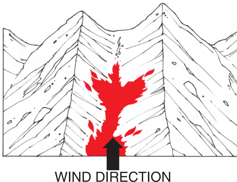
Illustration 1.14 The chimney effect
