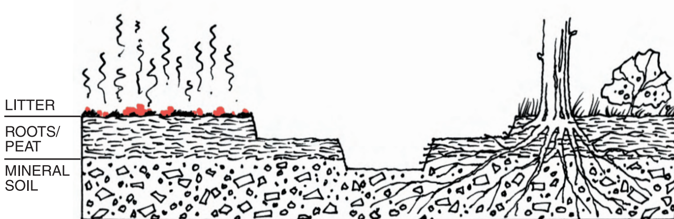
Illustration 3.3 Fireline construction - Cut / separate fuels and smouldering fire
